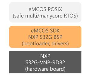
The new BSP ensures that the development of functionally safe and high-performance POSIX systems based on multi/manycore SoCs can begin immediately. The POSIX interface is vital because it means porting an application from Linux to the real-time eMCOS POSIX is a much more straightforward process.
